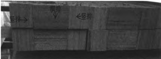
图 2 “竖-横-竖”优化结构 LVL 构件 Fig.2 LVL components assembled in vertical-horizontal-vertical directions
